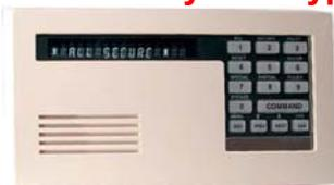
You have the 9000 series panel. To change the feature is command 55 and to add a code feature is command 56. To delete a code the feature is command 53.
