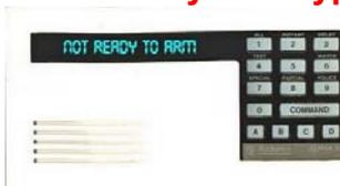
You have an 8112 series panel. To change existing codes will be either command 5 or 55 depending on your model number. Step 1: Press command followed by the number 5 or 55 button. The system will ask you to program the combination; it is looking for the old combination code first, so
