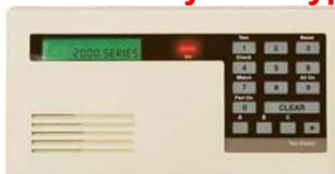
You have a 2212 series panel. The feature to change codes is to press the number 5 button. Step 1: Enter in the old code. Step 2: The system will ask you to enter in the new code; enter in the new code. Step 3: The system will ask you
